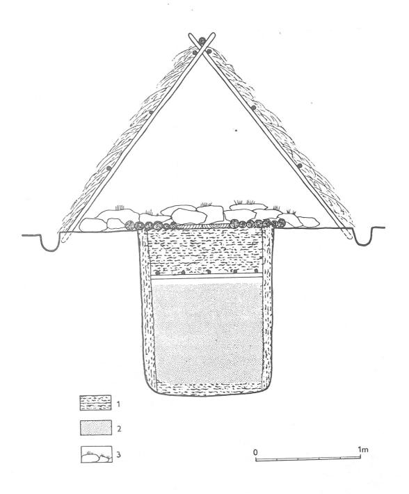
Fig. 2. Březno, district of Louny. Grain storage pit 71, reconstruction (a section). Key: 1 - straw; 2 - grain; 3 - sods.
