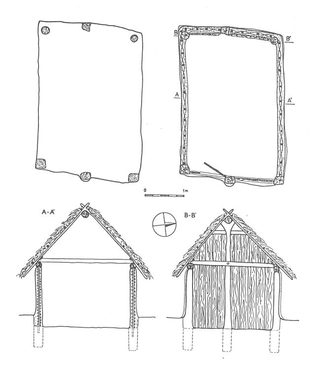
Fig. 1. Březno, district of Louny. House 13: 1 - the ground plan as found; 2 - the reconstructed ground plan; 3 - reconstruction of the building, section A-Á; 4 - reconstruction of the building, section B-B.
